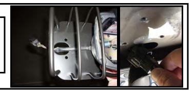
Step 9: Reinstall the tail light assembly and Euro Tail Light Guard to the original mounting holes using the factory hardware previously removed.
