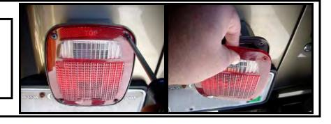
Step 3: Remove the 3 tail light assembly retaining bolts.
