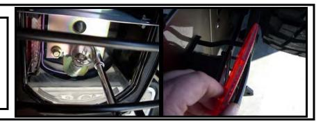
Step 11: Reinstall the four screws removed in step 1. Caution: Be careful not to over tighten these screws. Over tightening will crack the lens.
