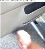
(5) Pop door panel back into place and reinstall screws removed in step (1). Repeat for other side.
