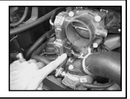
4. Place the gasket on the backside of the throttle body followed by the spacer (Logo up, rounded edge to the right). Place the supplied M6 bolts and washers through the front of the throttle body going through both the gasket and throttle body spacer.
