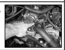
2. Loosen the 4, 8mm, bolts holding the throttle body to the intake manifold. Remove throttle body.
